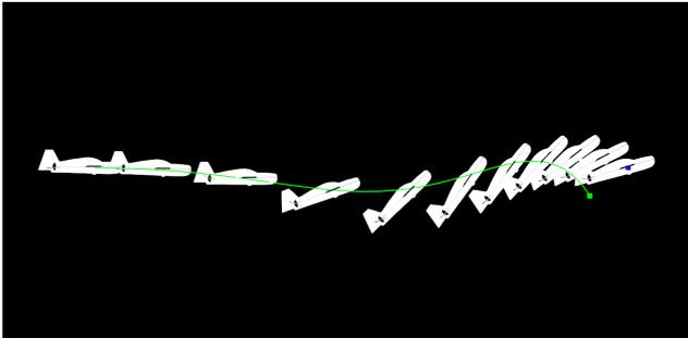
Fig. 3. Perching in the presence of unknown dynamics: Without adaptation. The vehicle center of mass (blue dot) overshoots the goal state (green dot).
